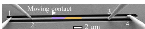
Figure 3. Electrical measurements across a GB. Current is supplied by needles 1 and 4, voltage is measured through needles 2 and 3. All needles are fixed at constant position except needle 2, which scans across the boundary. The EBSD-resolved grain map is laid on top of the GB region. (The tips of needles 3 and 4 are reshaped after electrostatic discharging while positioning them inside the SEM.).
