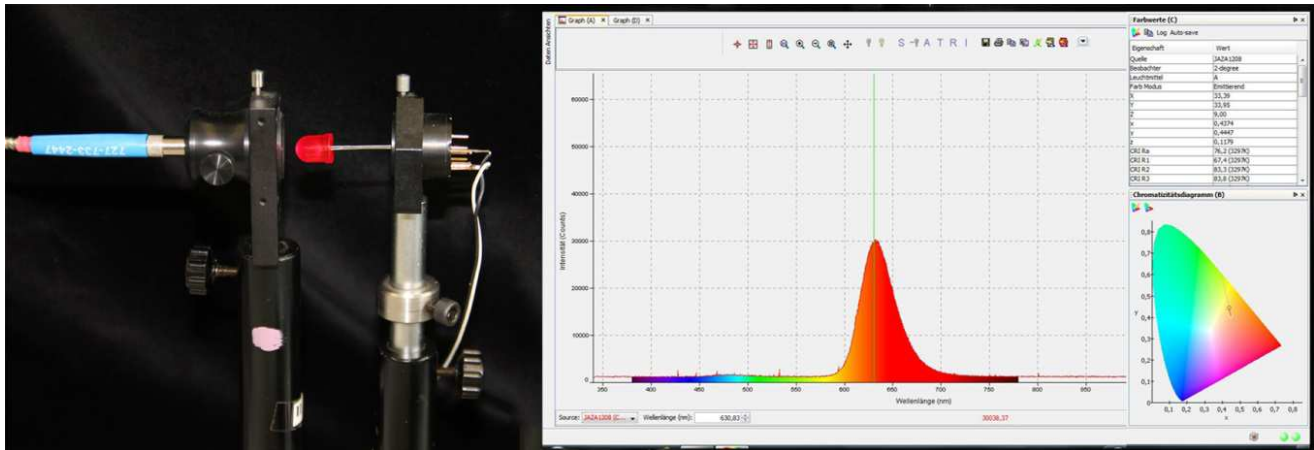
Figure 5. Measurement setup with a red colored LED and the corresponding result.
