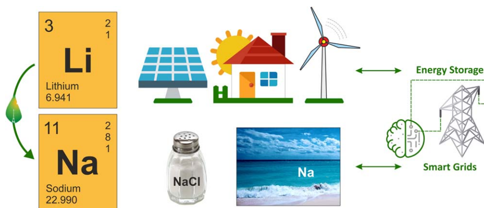
Figure 6. Schematic view of how moving from Li to Na based energy storage allows us to realize both local and decentralised energy ‘production’ (from, e.g. solar panels and wind power) as well as augmenting smart grids. It should be noted that such applications are possible even with today’s existing NIB technologies. Credits: Salt cellar: wikicommons: https://commons.wikimedia.org/wiki/File:Salt_shaker_on_white_background.jpg ; all other icons: from https://flaticon.com/ Credits: Solar energy icon with sun (Icon made by Smashicons perfect from www.flaticon.com ); house (Icon made by Roundicons from www.flaticon.com ); AI (Icon made by Eucalyp from www.flaticon.com ); grid (Icon made by Freepik from www.flaticon.com ). Photograph: salt availability as seen at a MuSR conference in Cancun, credit Martin Månsson.
