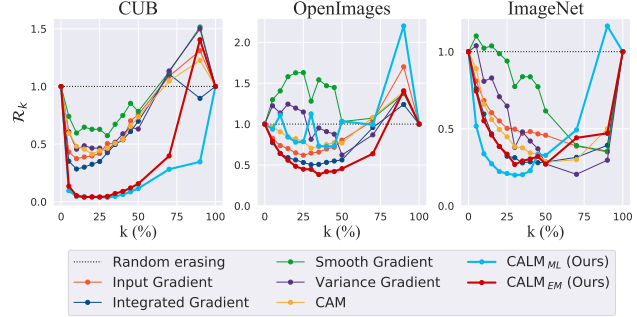
Figure 5. Remove-and-classify results. Classification accuracies of CNNs when k\% of pixels are erased according to the attribution values s_{hw} . We show the relative accuracies \mathcal{R}_k against the random-erasing baseline. Lower is better.
