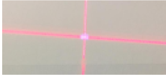
FIGURE 5.3: The laser level (red) are overlapped with the white synchrotron light produced in the bending magnets of the storage ring.
