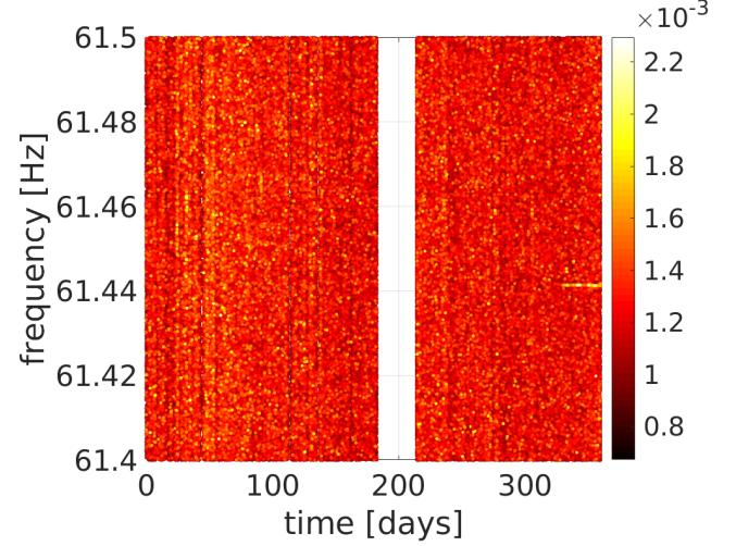
FIG. 16. Time-frequency peakmap of H1 data after the second follow-up stage (FU2) around the outlier with frequency  $\sim 61.44$  Hz. Time is measured in days since the starting of the run. A transient disturbance, starting from  $\sim 20$  days before the end of the run, is clearly visible. The color bar represents power spectrum in units of  $10^{-40}$  [1/Hz].
