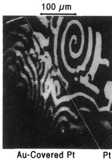
FIG. 3. Spiral waves on two adjacent sections of the Pt(110) surface from which the left one is covered by 0.05 ML Au. p_{O_2} = 4 \times 10^{-4} mbar, p_{CO} = 4.6 \times 10^{-5} mbar, T = 460 K.
