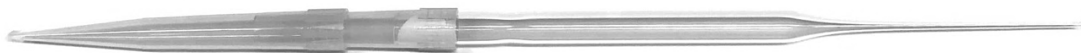
Figure 6: Odor stimulation cartridge. Pasteur pipet filled with filter paper at the top a covered with two tips and blocking out material.
