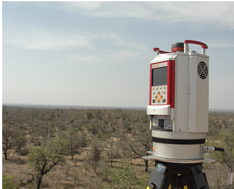
Figure 2.2: Riegl VZ-2000 terrestrial laser scanner at a terrestrial vantage point in KNP.
