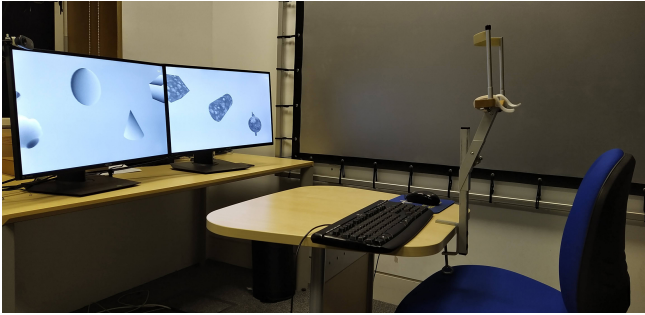
Fig. 14. Experiment Setup. We used a chinrest to keep viewer’s head at a fixed location.
