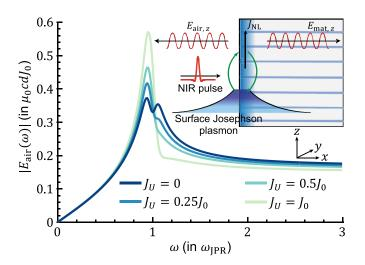
FIG. 2. Emission spectrum. We find that the outgoing radiation can be sharply peaked around  $\omega_{JPR}$  only in the presence of a nonzero umklapp photocurrent  $J_U \neq 0$ , Eq. (13). This umklapp component impulsively drives high momenta surface Josephson plasmons that can emit light [Fig. 1(b)]. Here we fixed  $A = 0.1\varepsilon_{\infty,c}$ .
