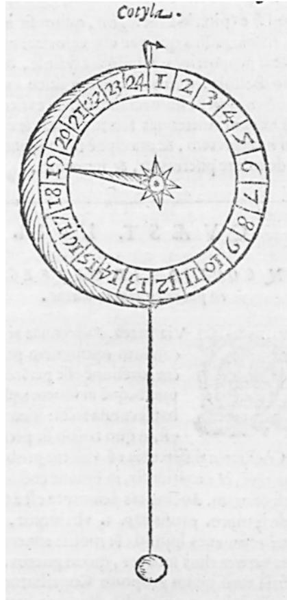
Hence, the design of the second beam type of *pulsilogium* improved the reliability of measurements by avoiding interferences that occurred in the first type due to its manual operation. Moreover, it enabled the physician to adjust the swing rate and to read the cord length while the pendulum was still in motion. Therefore, compared to the simple handheld *pulsilogium*, it provided more reliable measurements and its use must have been more convenient in medical practice.
