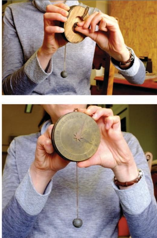
In his descriptions of the dial *pulsilogia*, Sanctorius indicated that the instruments measured both time and pulse frequency. It must therefore be assumed that they provided comparisons of degrees. In view of this, the bulky boxes as well as the movable dial might have been part of a special mechanism that allowed the two values to be registered simultaneously—a hypothesis that must, however, be further investigated (Sanctorius 1625: 222).
