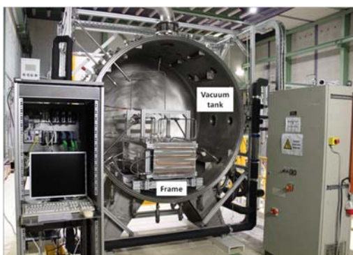
Fig. 5: Opened vacuum tank of the SIRHEX facility at KIT
