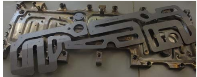
Fig. 2: Machined ground plate and machined sheets for the type 1h before welding) (Courtesy of Z-Innovation GmbH)
