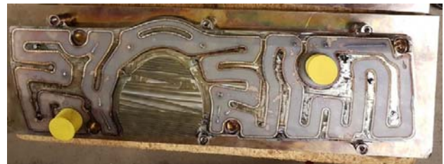
Fig. 3: Panels after electron beam welding of the likewise machined sheets to the ground plate. View from the back side of type 2v2 (prototype geometry) (Courtesy of Z-Innovation GmbH).
