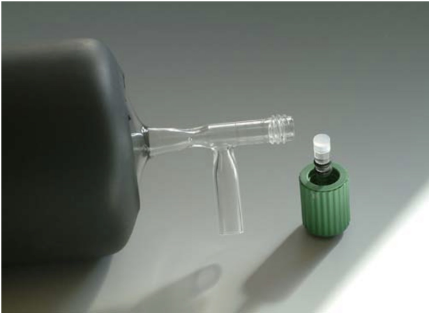
Figure 2: Sampling flask with PCTFE seal
