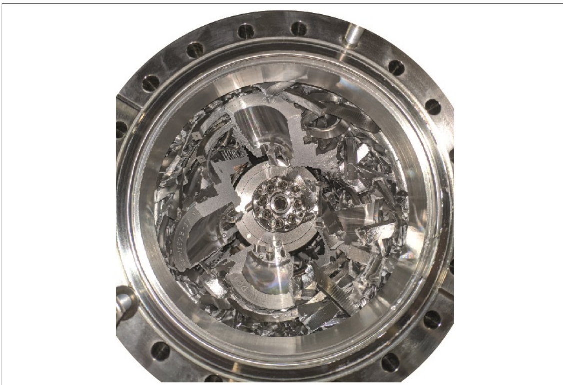
Figure 4.5: Sad left-overs of an Edwards STP-603 CF160 [75] turbo pump. Most pieces are completely stuck to the inner wall of the pump or to each other.
