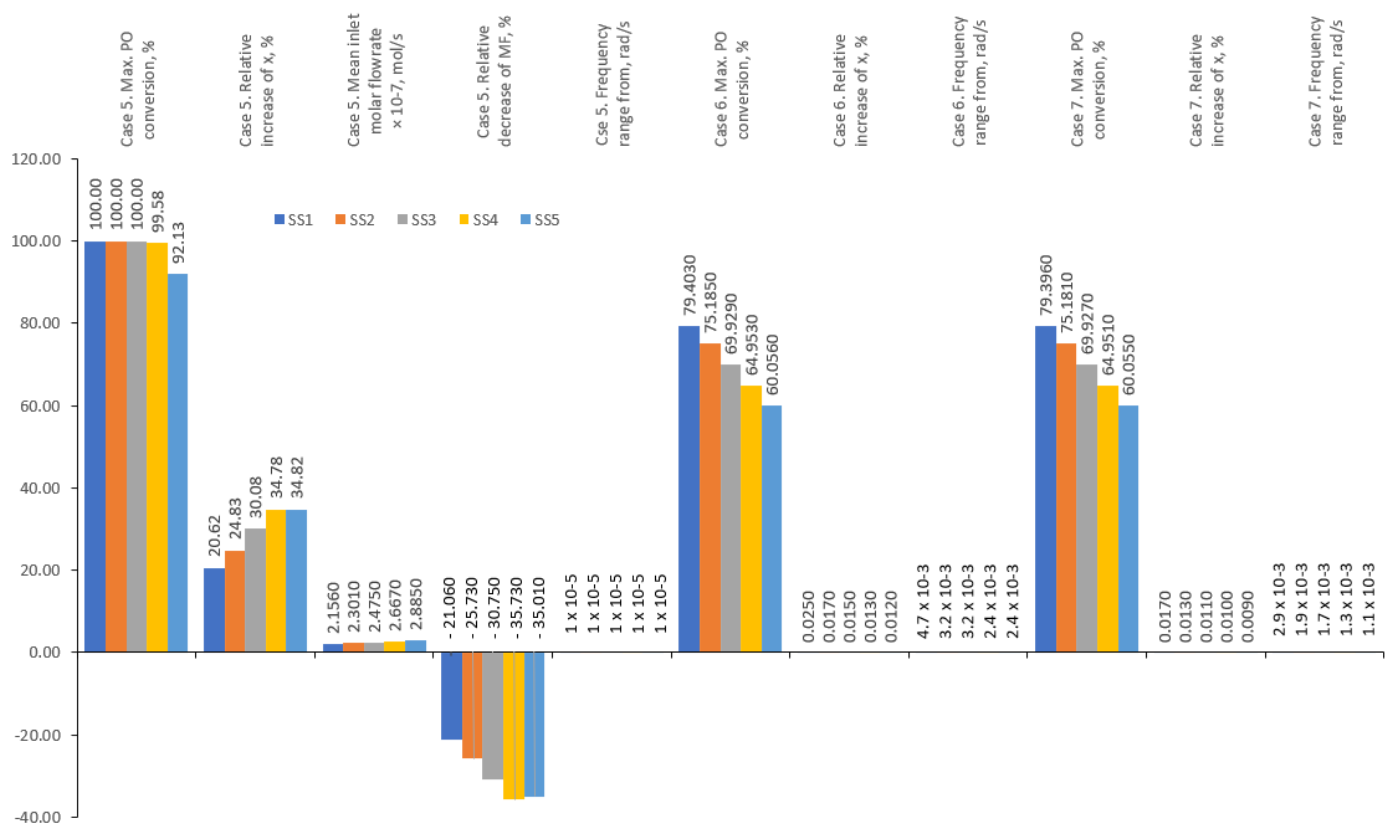
Figure 5. An overview of the possible improvement during simultaneous modulations of two input parameters for Case 5 (modulation of flowrate and acid molar fraction), Case 6 (temperature and acid molar fraction) and Case 7 (temperature and flowrate).
