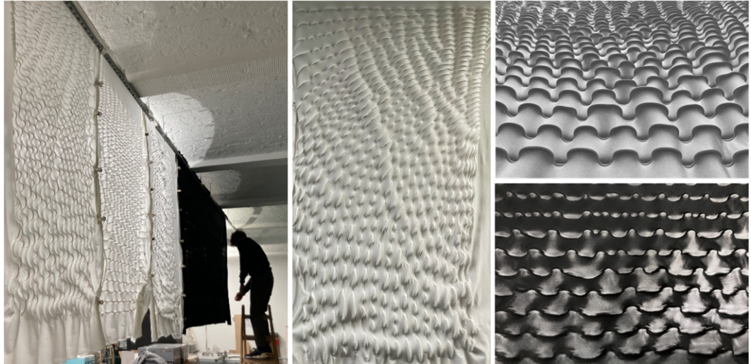
Figure 5. Self-shaping textile produced via manual deposition of polymeric adhesives into various geometric patterns of non-intersecting lines. The lines have approximately same thickness but variable spacing, orientation and number. Additional fabric tension due to gravity enrich the range of attainable surface textures with graded properties of translucency and shadow casting for an interior architectural setting.
