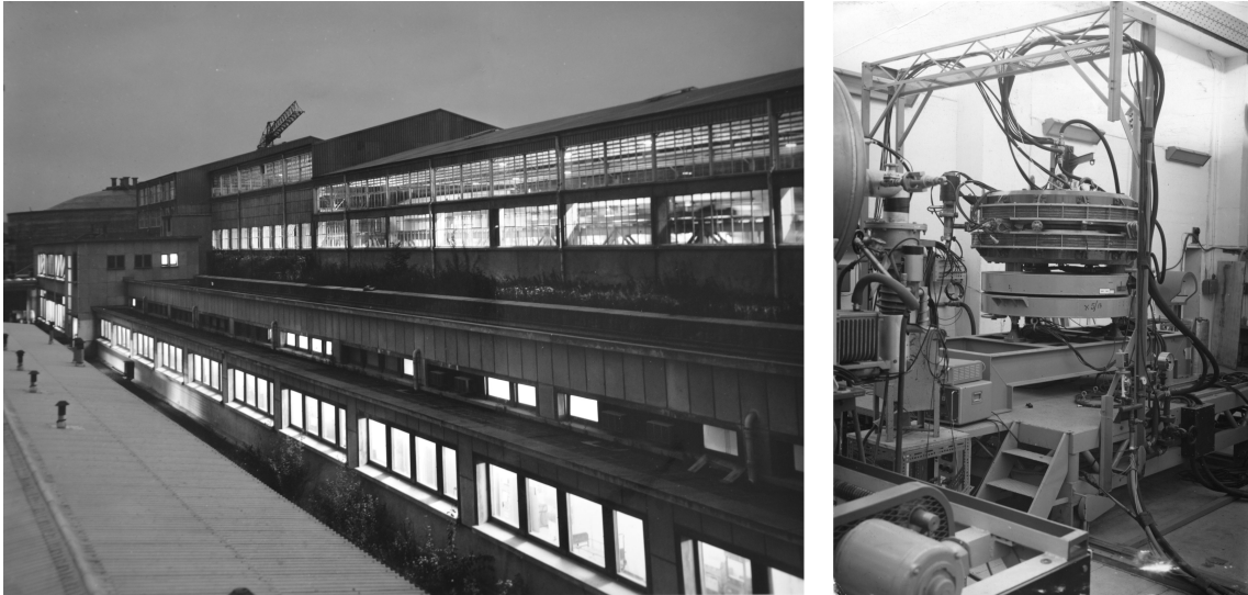
Figure 11: At left we show a photograph of the LAL Main building, housing the Linear Accelerator, and, at right AdA installed in Salle 500 at LAL, both courtesy of Jacques Haïssinski.
