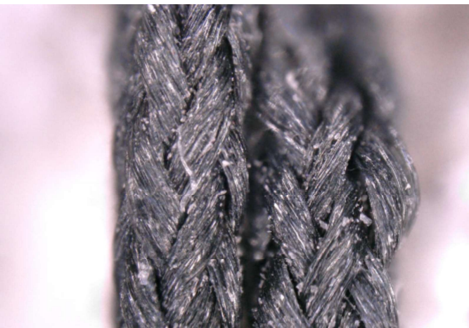
Figure 5. Black silk sutures at 300x magnification exhibiting silicone coating. Micrograph by Nicole Ong Yii Mei with Keyence VHX-5000. © Biomaterial Matters 2017
