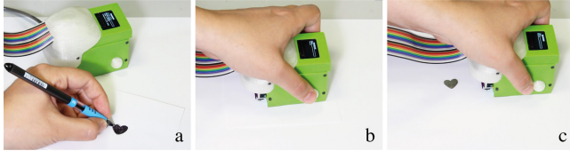
Figure 10: Scan & Print: a) Sketching custom design, b) scanning, c) and printing the design.
