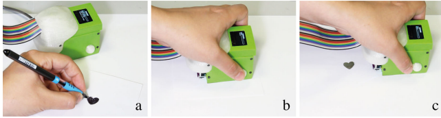
Figure 10: Scan & Print: a) Sketching custom design, b) scanning, c) and printing the design.
