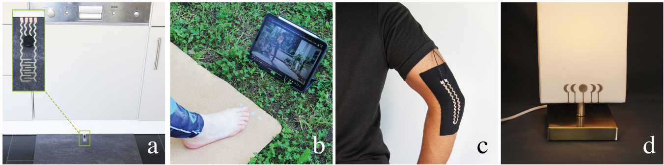
Figure 20: Application examples demonstrate the the practical feasibility and applicability of our technique on everyday surfaces: a) moisture sensor on a floor tile, b) interactive yoga mat, c) wearable stretch sensor on kinesiology tape, and c) capacitive slider on a table lamp.
