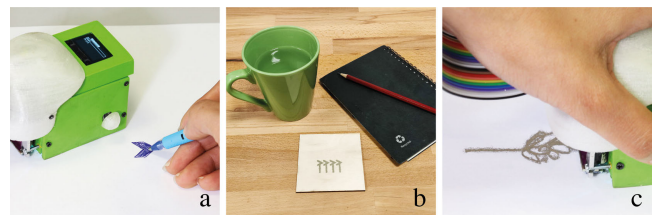
Figure 21: Images from user study: (a) drawing a customised electrode to scan & print, (b) Printed design based on hand-drawn electrode. (c) free form sketching.
