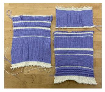
Figure 4: Samples of different rib structures added to the fullknit to provide indication of electrode sites.
