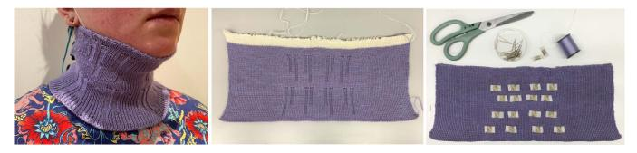
Figure 1: The *Singing Knit*, worn by Reed (left). Alternating ribbing on the outside of the collar highlights the position of the muscles and electrode placements (middle). Fabric electrodes made from zebra jersey are stitched by hand into the correct locations (right).
