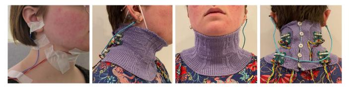
Figure 11: Reed wearing the completed knit collar, showing the knit's form on the neck compared to the original EMG setup.
