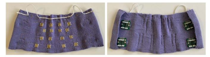
Figure 10: Amendments made to the collar: additional elastic is added to the inside of the collar to hold it up around the chin and provide support with straps around the ears (left). The excess fabric is folded over on the back to ensure a tight fit (right); these ends will be joined once the collar is on the wearer.
