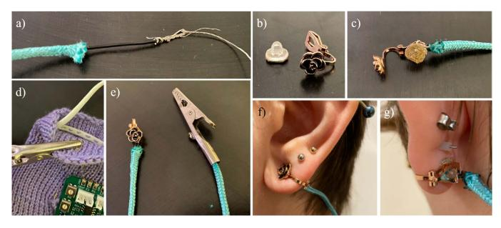
Figure 9: The construction of the earring reference electrode, starting with the cabling (a), stitching the conductive fabric to the earring pad (b-c), and securing the electrode to the collar and reference inputs (d) for a complete wearable (e). Reed wears the the electrode as part of their normal jewelry (f, g).
