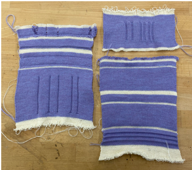
Figure 4: Samples of different rib structures added to the full-knit to provide indication of electrode sites.
