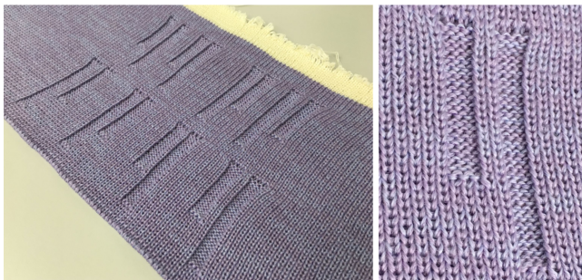
Figure 5: The ribbing added to the collar body, providing a visual for the muscles and electrodes situated on the inside of the collar.
