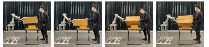
Fig. 6. Experiment results of the collaborative tasks. The human actors were performing lifting, pushing, clockwise rotating, and counter-clockwise rotating from left to right.
