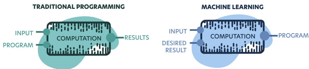
Figure 1.1: Schematic representation of the difference between the traditional programming, based on the algorithmic approach, and the experience-based/data-driven approach, which is the backbone of the ML paradigm. The ML paradigm is the first step toward learning abstractions by computers through the extraction of common features from data.
