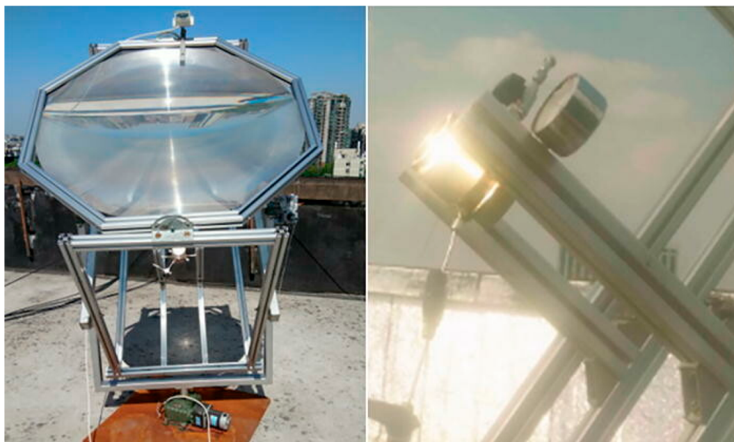
Figure 4. Solar concentrator setup for batch photocatalytic CO 2 reduction (left) and close up of its reaction chamber (right). Reprinted with permission from ref 52. Copyright 2021. AIP Publishing.
