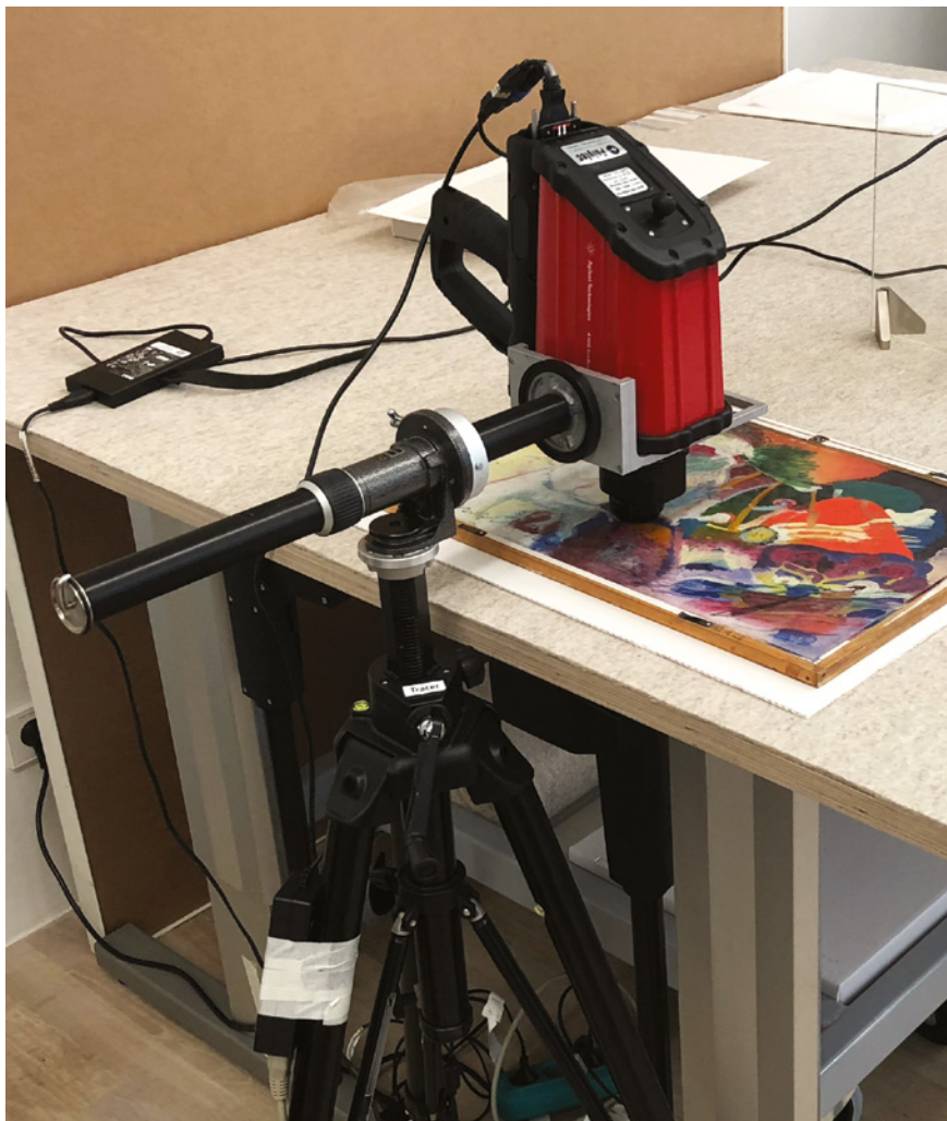
FIGURE 42 FTIR Spectroscopy in diffuse mode (DRIFTS) ExoScan spectrometer (A2 Technologies)
