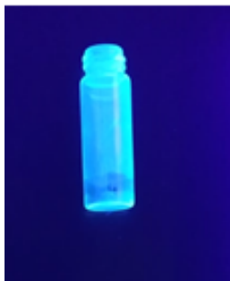
Figure S5 - Carbon nitride coated Glass vial coated with the CN film under UV light. Bottom part of the vial was scratched due to mechanical friction caused by the magnetic stirrer used during the reaction
