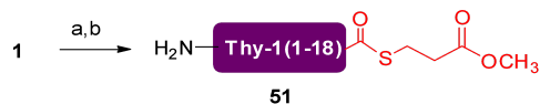
Scheme 63 - Thiolyis of fragment 1 . Conditiond: a) Gdn*HCl 6M, Na 2 HPO 4 0.2 M (pH 3.0 – 3.2), NaNO 2 , -10°C 20 minutes; b) MMP, 25 °C, pH to 6.7 – 6.9, 5 min.
