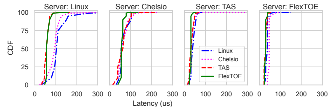
Figure 9. Latency of different server-client combinations.
