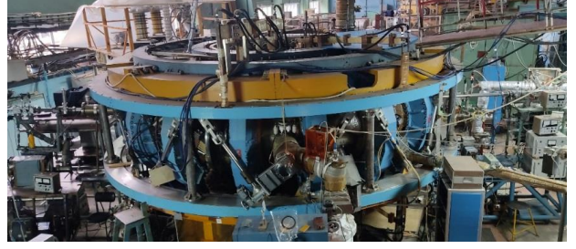
Fig. 1. General view of stellarator Uragan-2M.
