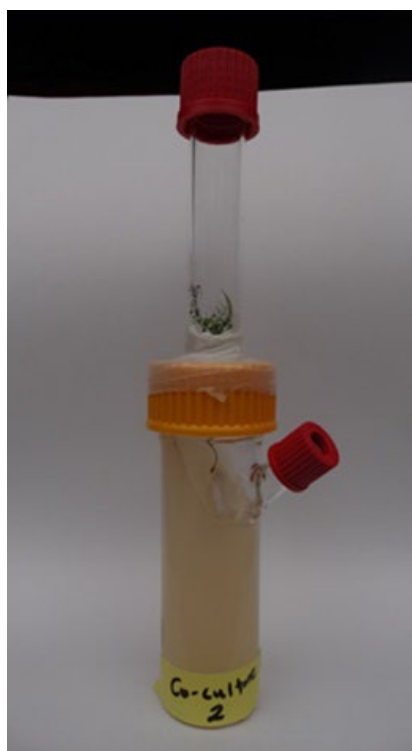
Figure 1. Experimental set up for the sampling of root volatile organic compounds. The green tree parts are visible and separated from the below-surface root fungus system, where sampling was made possible through the inlet Teflon cap visible at the right.
