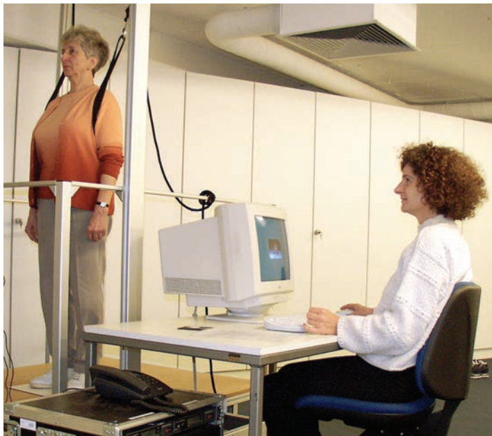
Figure 2. Dynamic posturography. Balance performance on the moving platform can be assessed while participants simultaneously perform a cognitive task.
