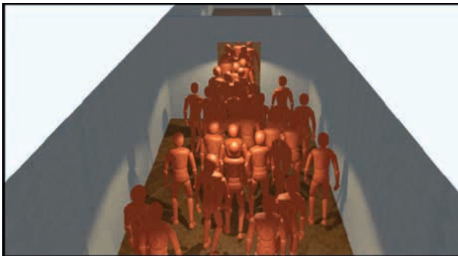
Figure 10. Snapshot of the virtual environment during a simple evacuation procedure (Moussaïd et al., 2016). Each avatar in this snapshot was controlled by a real participant who had a first-person view of the surrounding environment.
