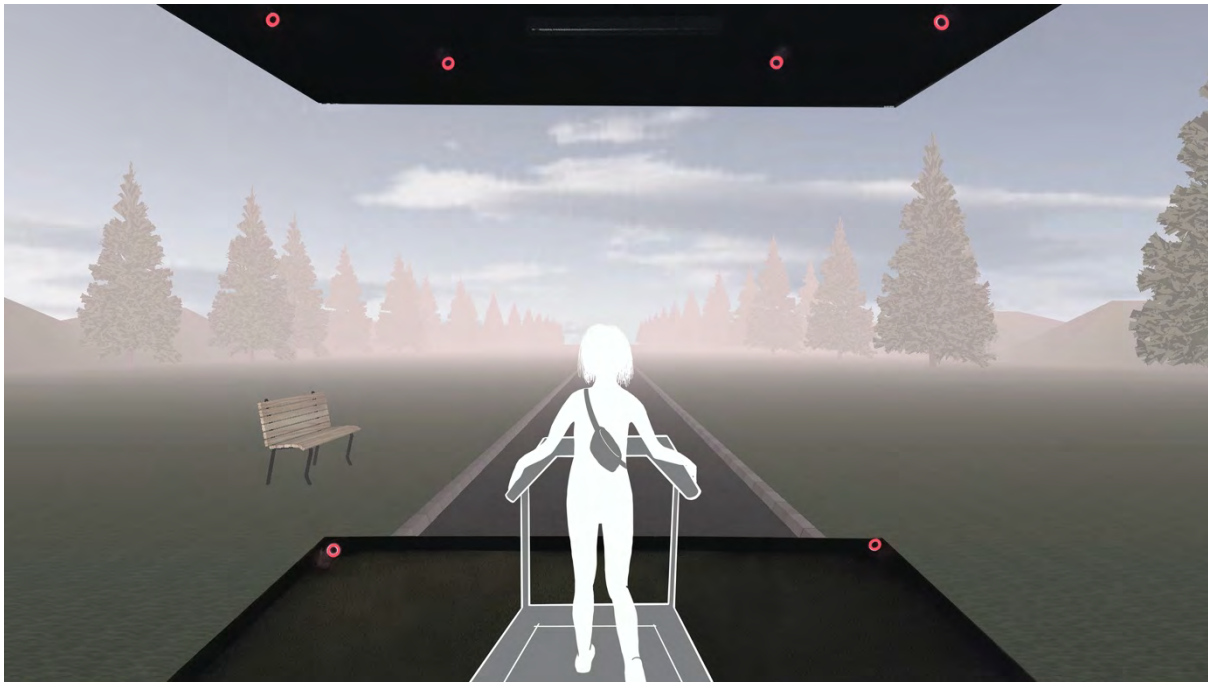
Figure 2: Illustration of the CAVE setup with its three screens. Participants walked on a treadmill through a variety of dynamic virtual environments, encountering both landmark (here: a bench) and endpoint objects along the way while their eye movements were continuously tracked and recorded. A subset of the infrared cameras is marked red.
