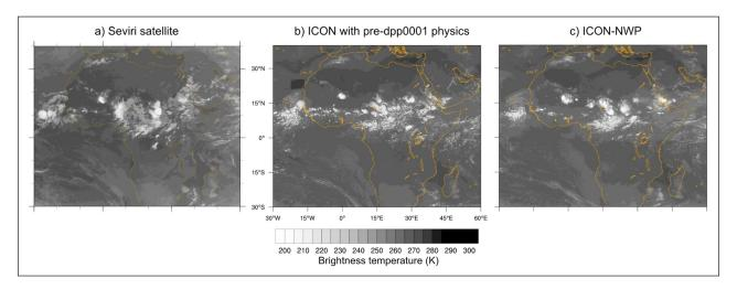
**Figure 6** Comparison of infrared brightness temperature observed from the Seviri weather satellite **(a)**, with 12-hour initialised runs from an early version of ICON-Sapphire with diagnostic cloud micro physics **(b)**, and with the numerical weather prediction (NWP) physics package that includes prognostic cloud micro physics used by the German Weather Service (DWD) **(c)**.
