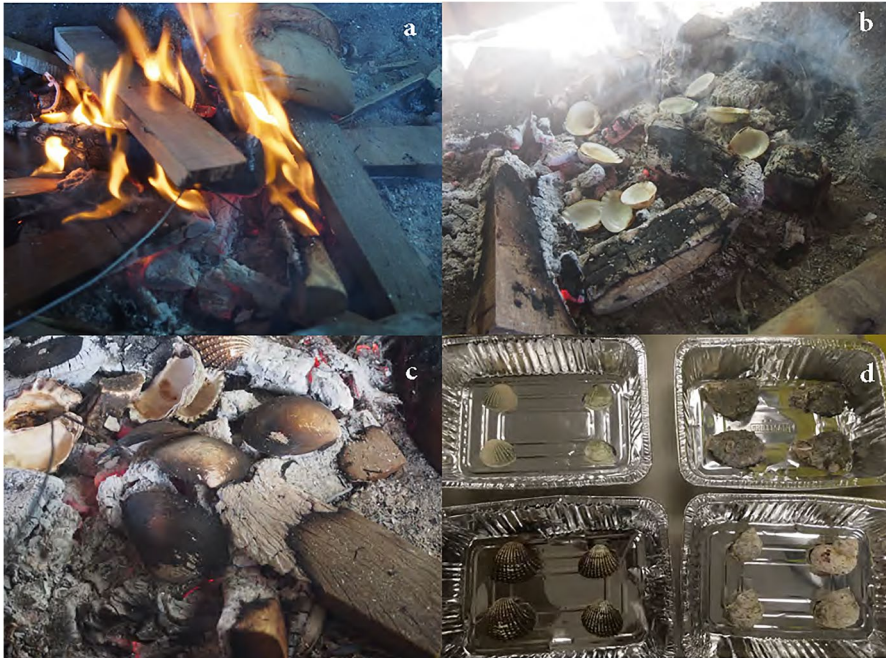
Fig. 4 Progress photos during burning and heating experiment. a Showing fire for flame method, b and c showing coal methods, d showing samples before inserting into muffle furnace for heating method
