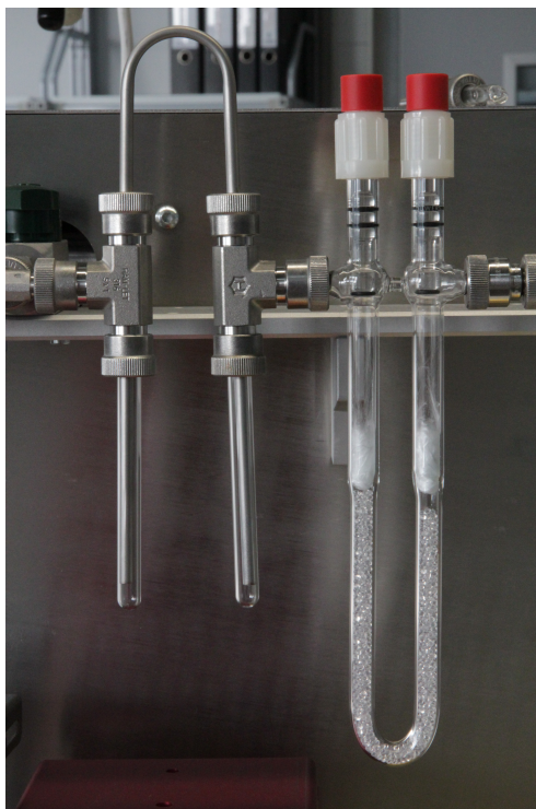
FIGURE 2.8: Picture of two types of U-shaped glass traps. Picture taken in the 14 C-Analytik laboratory at MPI-BGC, Jena. The version on the left side is identical to the ones used in pre-existent purification lines at LAC-UFF. The glass trap with pellets inside (right side) is the version used in GASPS. The pellets increase the surface area with the gas sample.
