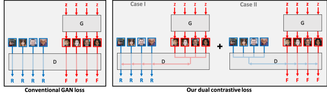
Figure 2. Comparisons between the diagram of conventional GAN loss and diagram of our dual contrastive loss. Our contrastive loss in Case I aims at teaching the discriminator to disassociate a single real image (R) against a batch of generated images (F). Dually in Case II, the discriminator learns to disassociate a single generated image against a batch of real images.
