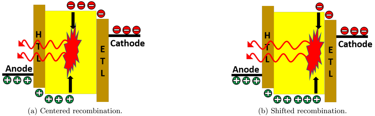
Figure 4.14: Centered and shifted recombination in OLEDs due to balanced and unbalanced charge transport.
