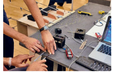
Fig. 3a (right): Motors and flex sensors are connected to the steel wires of the lattice.
