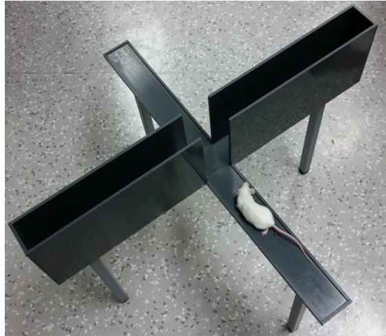
Figure 2.2: Elevated plus-maze (EPM) test. The experimental setup of the EPM test consisted of two opposing brightly lit open arms and two opposing dimly lit closed arms.
