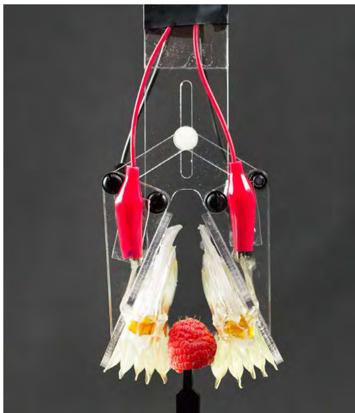
Example of a soft robotic hand, whose design is based on HASEL actuators. The gripper is gentle enough to handle raspberries without crushing them.
