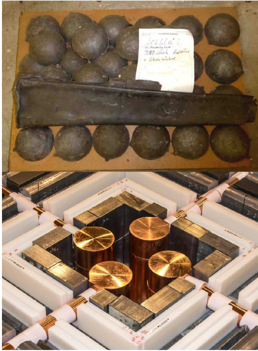
Fig. 14 Top: Old Pb half-spheres from the Freiburg Minster, low in ^{210}\text{Pb} activity; Bottom: Innermost Pb layer of the CONUS shield consisting among others of the Pb bricks melted from the Freiburg Minster Pb.
