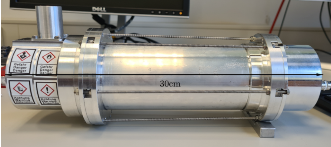
Figure 1: The picture shows the scintillator module used to measure the relative light yield and pulse shape discrimination capabilities of the liquids.
