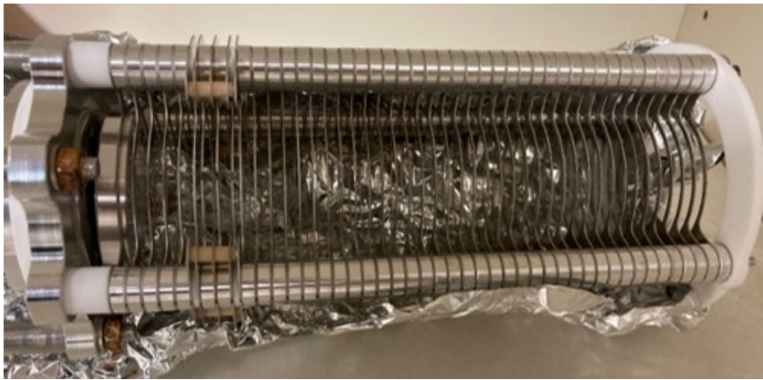
Figure B.1: Construction of the transparent Penning trap
