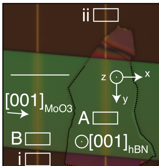
Figure S7 | Microscope image of the device used in experiments with Au launchers. The white scale bar is about 34 \mu\text{m} in length (See text for details).
