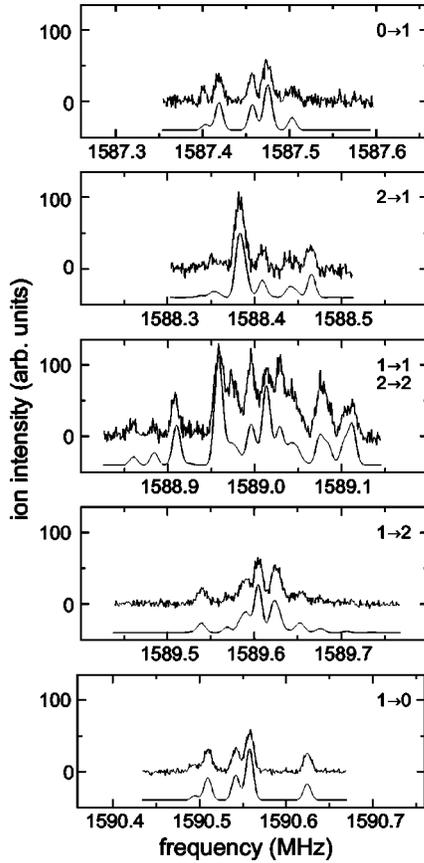
FIG. 3. The five main  $F'_1 \rightarrow F''_1$  transitions in the microwave spectrum of  $^{14}\text{ND}_3$ , recorded with a spectral resolution of 10 kHz. The upper trace in each of the graphs shows the experimental spectrum while the lower trace is the simulated spectrum, using the parameters in the Hamiltonian as obtained from the best fit.
