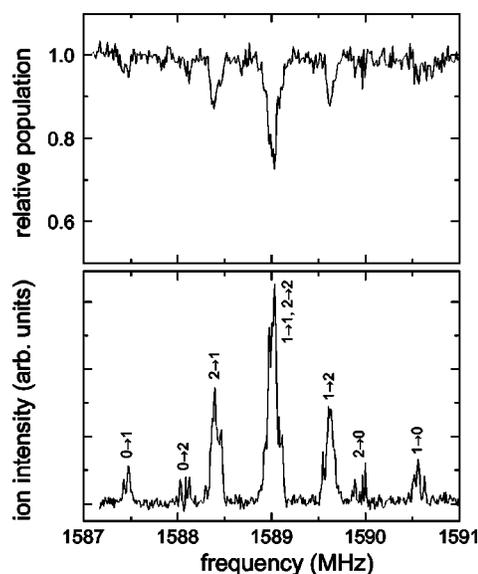
FIG. 2. Pure inversion spectrum of  $^{14}\text{ND}_3$  ( $|J, K\rangle = |1, 1\rangle$ ), measured by probing both the upper component (upper trace) and the lower component (lower trace) of the inversion doublet. The spectra are recorded at high microwave powers (1 mW) and are power broadened. Assignment of the main  $F'_1 \rightarrow F''_1$  features is given in the spectrum.
