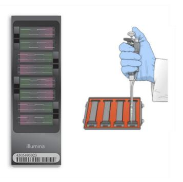
**Figure 6. Illumina MethylationEPIC BeadChip setup.** Left: One chip with 8 array slots. Right: Hybridization chamber in which samples are hybridized to EPIC BeadChips. Modified from http://emea.support.illumina.com/infinium-hd-methylation-guide-15019519-01.pdf.
