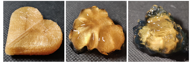
Fig. 11. The evolution of a printed object in undisturbed water. Water seeps into the material, forming a jelly-like substance. This interferes with our release model as the swelling impedes the free flow of water. Though the solution is constantly mixed during our dissolution measurements, here we avoid stirring to simulate local conditions where the flow is minimal.
